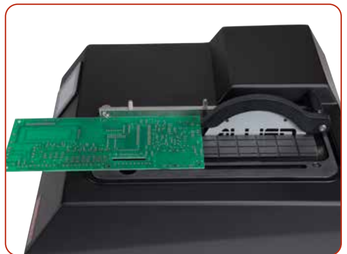
Adjustable table rip fence for measured/guided sectioning
